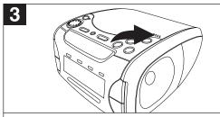
Open the CD compartment door by pressing the OPEN/CLOSE area. Insert a disc, label side up, onto the spindle and close the CD compartment door.
